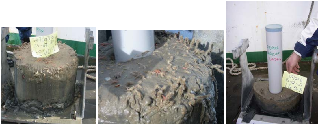
Figure 3: Boxcore of muddy sand sampled in the swale north (SV01, left and middle) and east (LG34a) of the dumping place B&W S1 (SV1). A lot of tubeworms were encountered in SV01.
