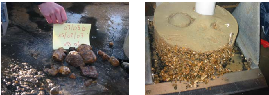
Figure 5: Boxcore of gravels, taken in the swale between the Oostdijk and the Buiten Ratel (VB06). Boxcore of shell debris, shells and gravels, sampled in the swale between the Buiten Ratel and the Kwintebank (VB02b).
