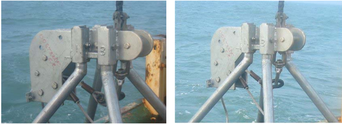
Cable of the arm (onto which te bucket is attached) is stuck in the “knob” of the grab.
