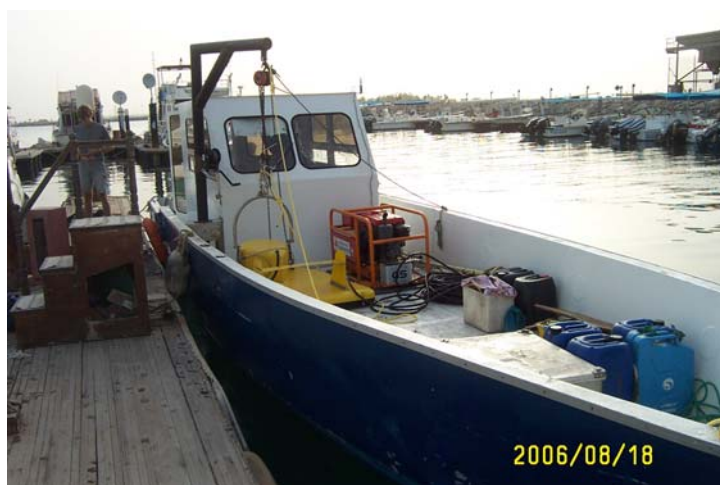
Figure 3. The support vessel needs to be of an adequate size but, as shown, a small half-decker may be adequate. Note that the deck has ample room for the towfish and an electrical power supply.
