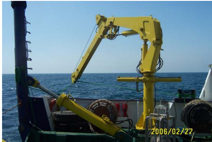
Figure 2. Example of an appropriate crane for towing.
