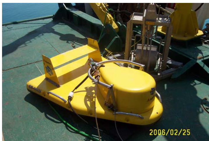
Figure 1. Towfish of a Chirp sub-bottom profiler system (weighing 190 kg).
