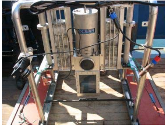
Figure 4. SPI equipment fitted with a small video-camera (right) and lighting system (left) enabling the SPI to be used more selectively (source: Cefas).
