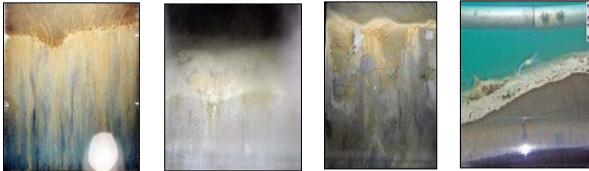
Figure 6. Examples of obscured SPI images. Left to right: flare from flashlight, suspended sediment in water reducing visibility, smearing on the face plate, obstructions in the image (photos by R. Diaz).
